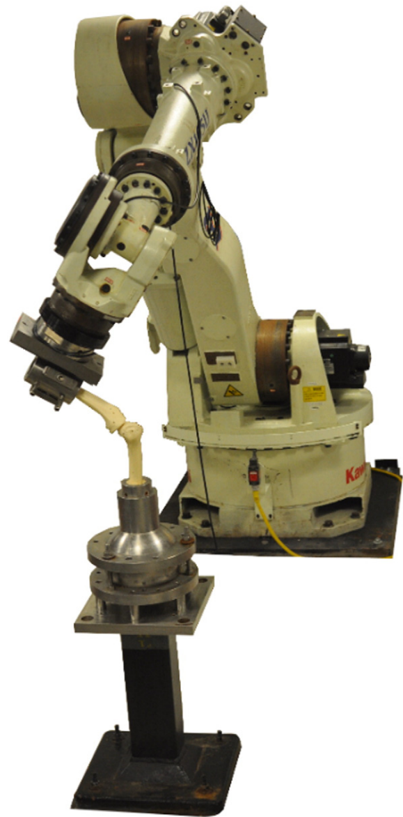
Figure 1. Cadaver knees were loaded using a robotic manipulator equipped with a universal force-moment sensor.
